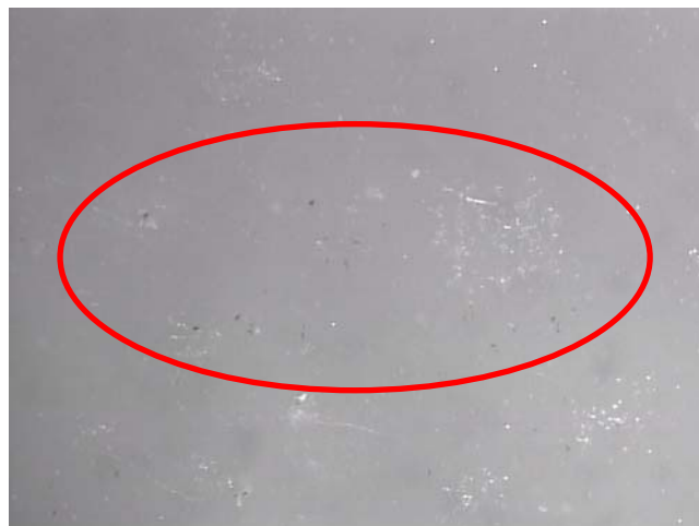
Photo 2: Material Würth Acetatsilikon Lebensmittel , color transparent/ white after an incubation period of 28 days with low fungal growth (at a magnification of x 50)
